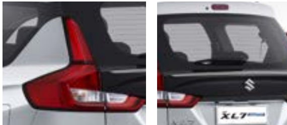
BOLD LED REAR COMBINATION LAMP WITH LIGHT GUIDES***
